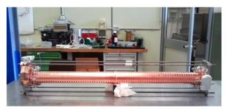
Figure 4: The two halves of one C-band section before the final brazing.
