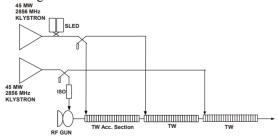
Figure 1: the SPARC photoinjector present layout.
