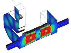
Figure 3: The waveguide beam-pipe coupling.
