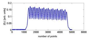
Figure 5: RF field profile of half C-band section.
