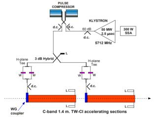
Figure 7: Layout of the SPARC C-band system
