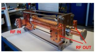
Figure 2: The C-band prototype tested at KEK.
