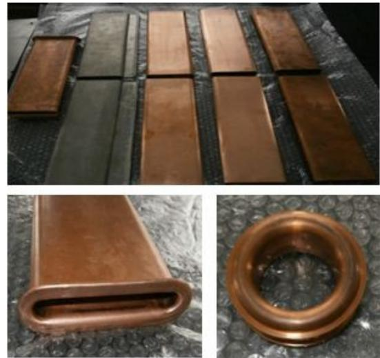
Figure 8: Parts of copper CH cavity.
