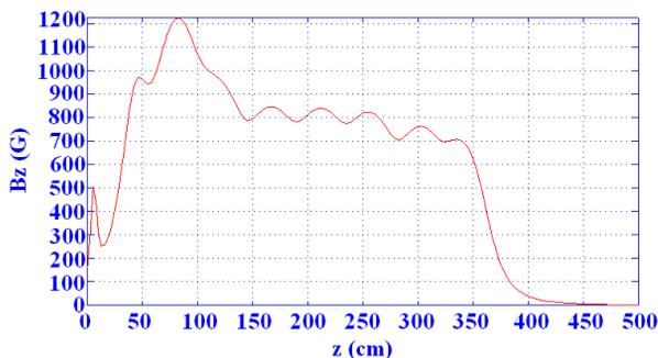
Figure 4: The solenoid magnetic field distribution along the 10 MeV / 40 kW linac.
