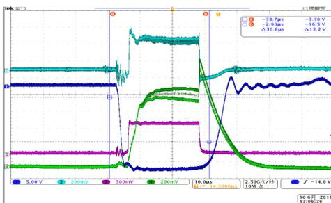
Figure 9: Machine status: blue line is the modulator high voltage waveform, turquoise the beam current from BCT, pink forward RF, and green reflected RF. Time-scale is 10  $\mu$ s/division.
