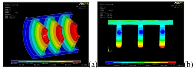
Figure 5: ANSYS results for the structure heating under the design parameters: (a) the iris temperature rise; (b) the structure deformation.
