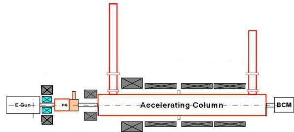
Figure 1: The schematic of the L-band linac.
