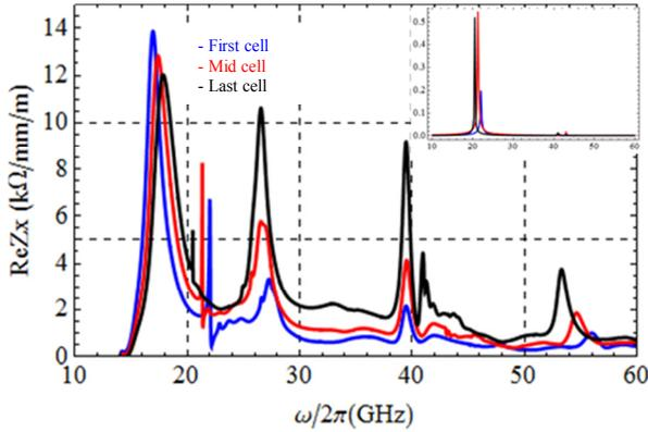
Figure 2: Transverse impedance in single cells of CLIC AS. Impedance for a window of 3m to 7m wake-length is shown inset.
