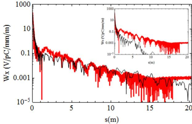
Figure 3: Comparison of the envelope of transverse wakefield in CLIC AS using GdfidL (red curve) and reconstruction using single cell modes (black curve). Inset compares the reconstruction excluding the 21 GHz mode.
