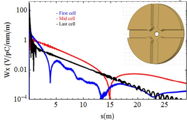
Figure 1: Envelope of transverse wakefield in single cells of CLIC AS.
