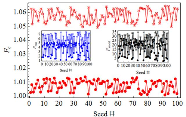
Figure 6: Amplification parameters of CLIC AS with random errors of +/- 1% in bunch spacing.
