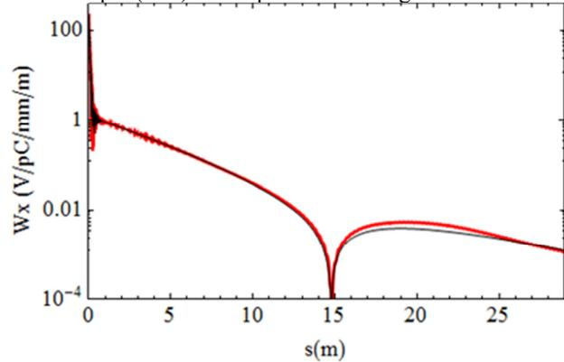
Figure 4: Reconstruction of wakefield in the middle cell using modal sum method. The black curve represents reconstruction, the coloured curve GdfidL simulation.
