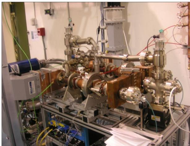
Figure 2: The power coupler test set up.
