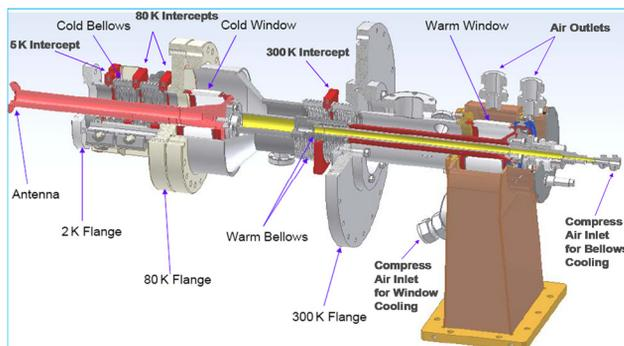
Figure 1: The CPI coupler is based on the Cornell 60 kW TTF-III coupler design.
