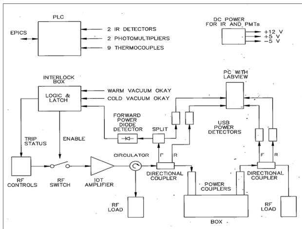
Figure 3: A block diagram of the RF set up.
