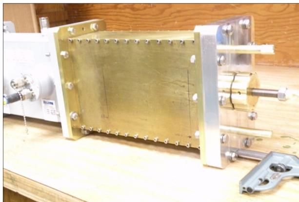
Figure 5: Movable WR650 waveguide short
