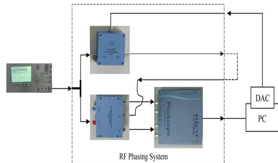
Figure 7: Self-test for RF phase stability system
