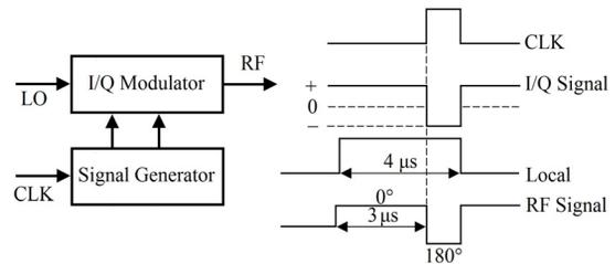
Figure 3: Schematics of the 180° phase reversal system
