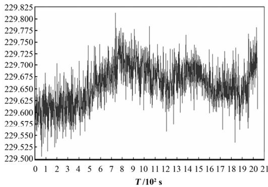
Figure 8: Phase measurement resolution
