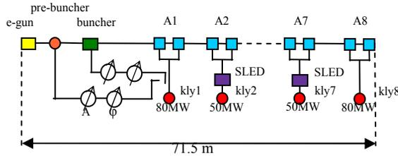
Figure 1: 800MeV Linac layout
