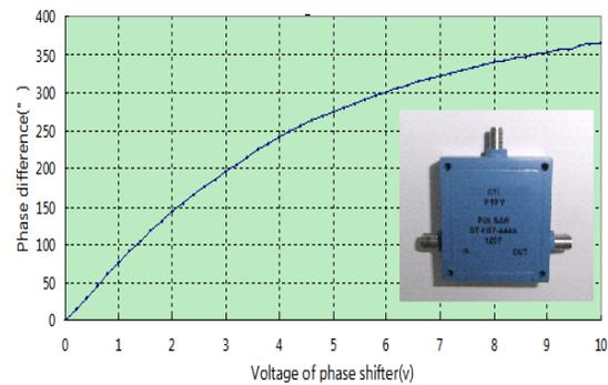
Figure 6: Phase shift vs control voltage
