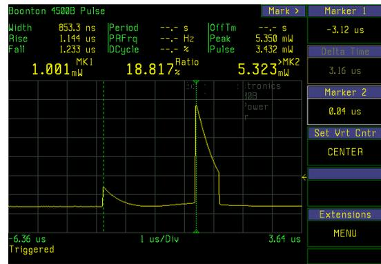
Figure 2: SLED RF output profile
