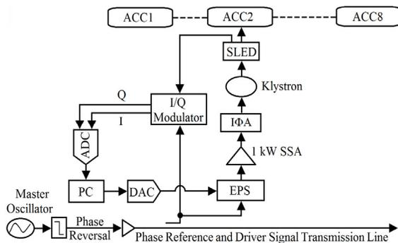
Figure 5: Diagram of phase stability system
