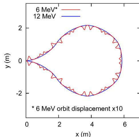
Figure 3: Layout of the 6 and 12 MeV reference orbits.
