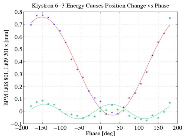
Figure 3: The phase of klystron 6-3 was varied and the resulting downstream orbit observed. At BPM Li09 201 it was up to 800  $\mu\text{m}$  and in phase with acceleration, two BPMs earlier, near the zero-crossing, a 100  $\mu\text{m}$  2<sup>nd</sup> harmonic-like effect was seen.
