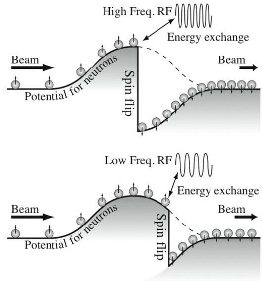
Figure 2: Control of deceleration by using AFP spin flipper with variable frequency RF. Top and bottom shows large and small deceleration respectively.
