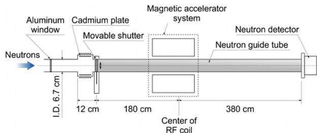
Figure 7: Experimental setup. Neutron accelerator is installed in the middle of the guide tube. The RF and data acquisition systems are synchronized with the shutter operation.
