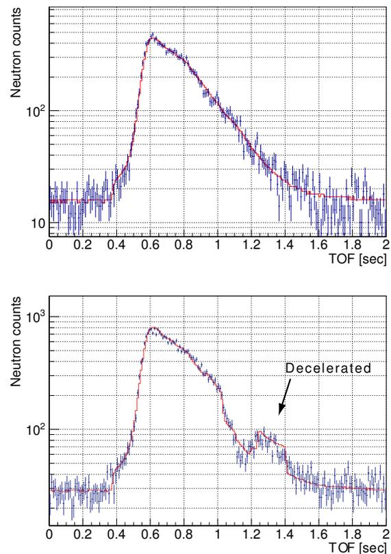
Figure 8: Neutron TOF spectra. Top and bottom show the case of RF OFF and ON respectively. Lines show the simulations.
