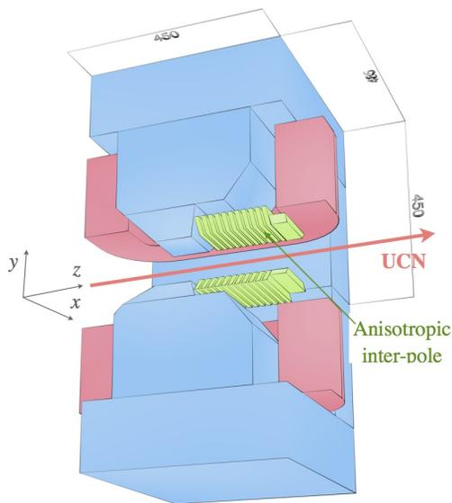
Figure 4: Magnet with anisotropic inter-poles.
