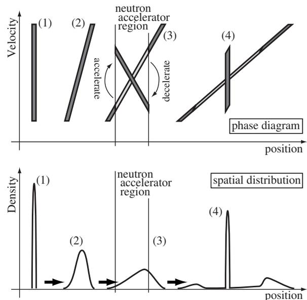
Figure 1: Concept of space-time focusing by using neutron accelerator. (1) Neutrons are generated as a pulse. (2) Neutrons spread spatially during transport. (3) Neutrons are accelerated/decelerated properly. (4) Some neutrons are focused at the experimental position. This figure illustrates the behavior of polarized neutrons.
