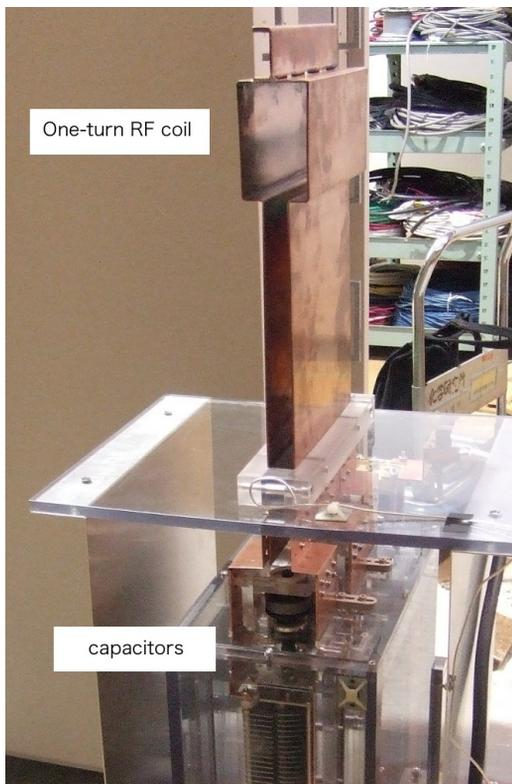
Figure 5: One-turn coil for RF and capacitors.
