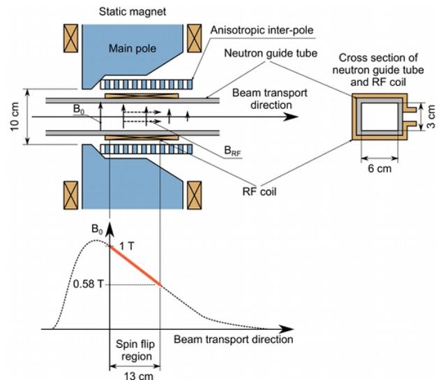
Figure 3: Closeup view of the magnetic accelerator system together with the illustration of the magnetic field gradient in the beam transport direction.
