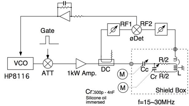
Figure 6: Electric circuit to match the resonance condition of RF.
