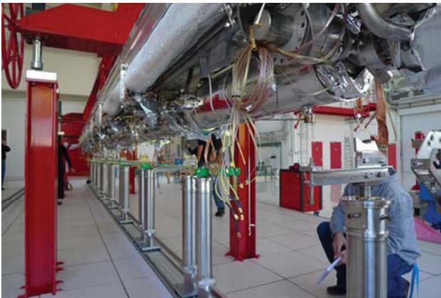
Figure 3: Assembly of the cold mass at CEA Saclay.
