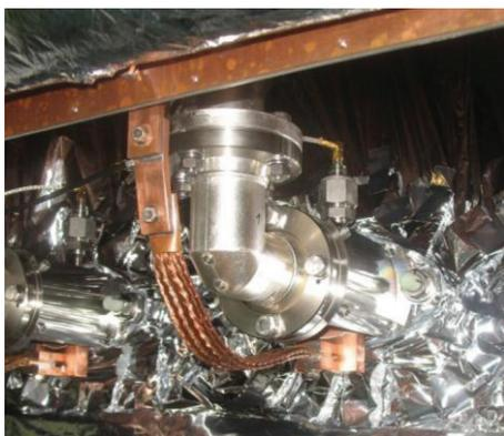
Figure 7: Coupler elbow section (Fig. 6) photo with the cooling strip connected to the 70 K thermal shield.
