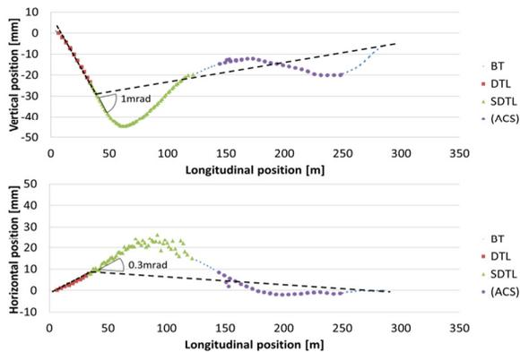
Figure 3: Displacement of the accelerator components after the earthquake (dots) and target realignment line (dashed lines).
