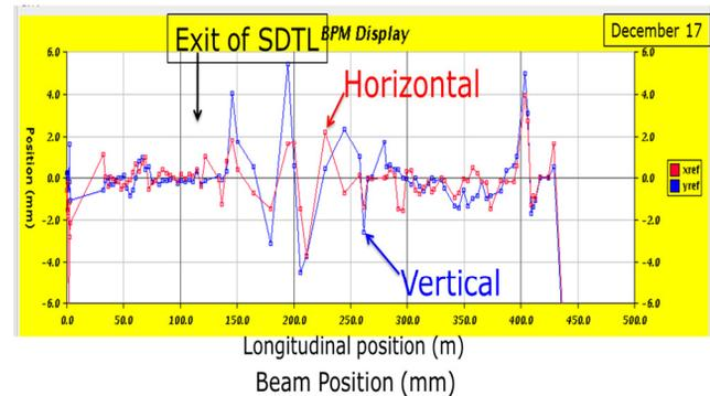
Figure 5: Beam position at the minimum beam loss condition on December 17, 2011.
