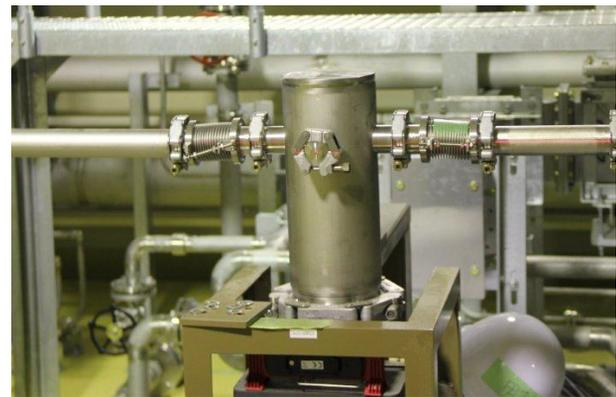
Figure 6: Displacement of the box. Deformed bellows with a red laser level marker line are shown.
