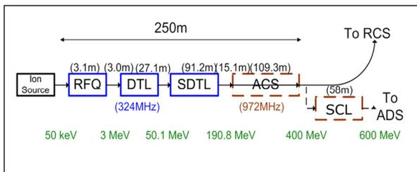
Figure 1: The structure of the J-PARC linac.
