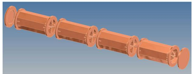
Figure 3: Engineering model of the 4-segment 4-vane RFQ.
