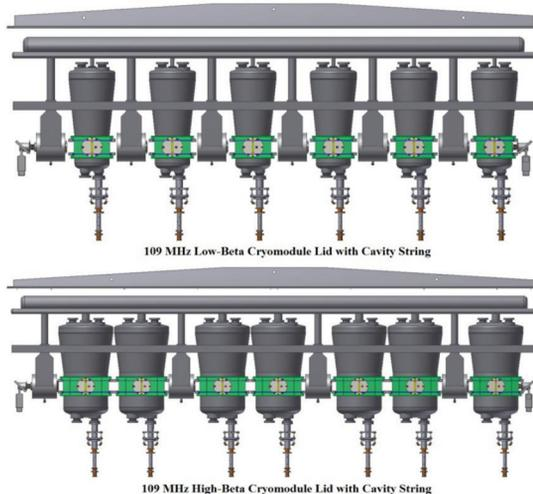
Figure 7: The 109 MHz superconducting modules, low- $\beta$  (top) and high  $\beta$  (bottom) lattice design.
