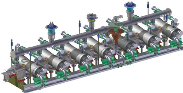
Figure 5: 3D engineering model of the cavity-solenoid string attached to the cryostat lid. 176 HWR option.
