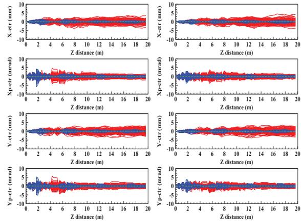
Figure 6: 176-MHz linac beam centroid motion-  $x, x', y, y'$  along the linac for 100 error simulations of 5-mA proton (left) and deuteron (right) beams simulated with  $10^5$  particles each, blue curves- with monitors and corrections scheme.
