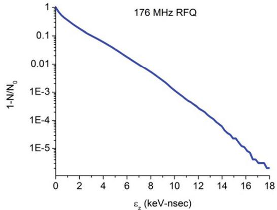
Figure 2: The relative number of particles located outside a given longitudinal emittance obtained by simulation of 200k particles with an input current of 5.5 mA.
