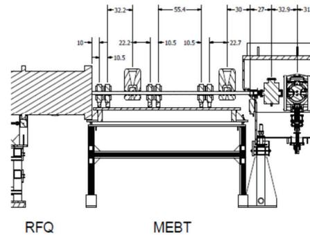
Figure 4: Medium energy beam transport (MEBT).
