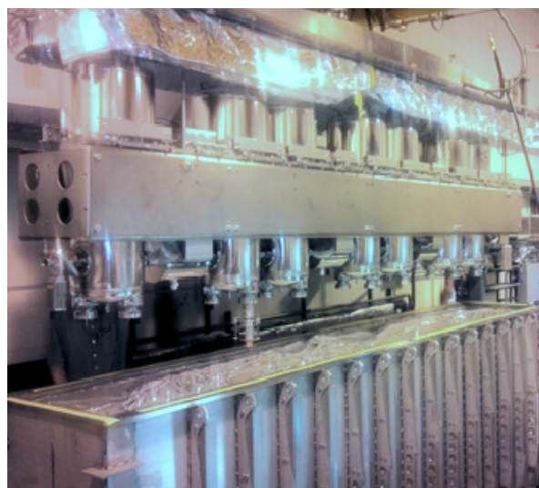
Figure 4: Cavity string is being lowered into the box vacuum vessel during mock assembly.
