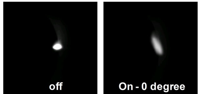
Figure 6: Beam on a scintillator screen with rf deflector off and with rf deflector on at 0 degrees.
