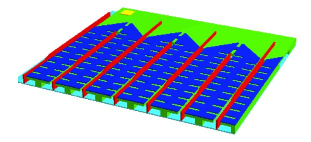
Coupling between adjacent folds cause dispersion, which limits bandwidth and/or maximum structure length. Typical max length is~.5m
