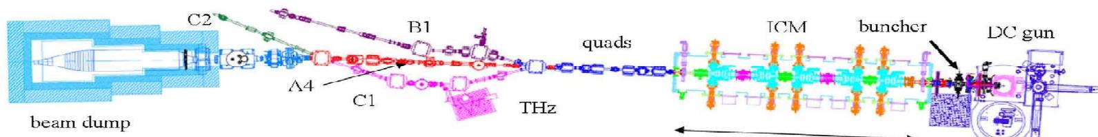
Figure 2: The layout of Cornell prototype ERL injector. Beam direction is to the left.
