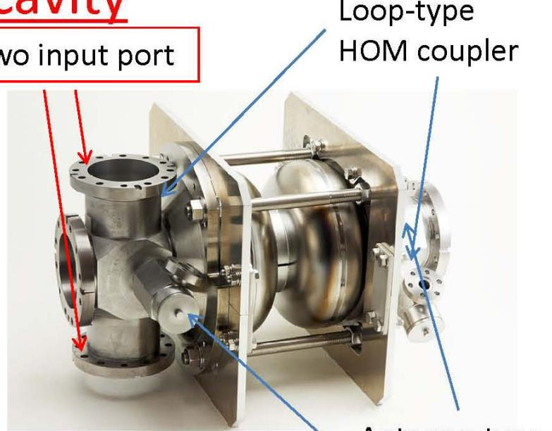
Basic cavity Parameters for Injector at KEK
