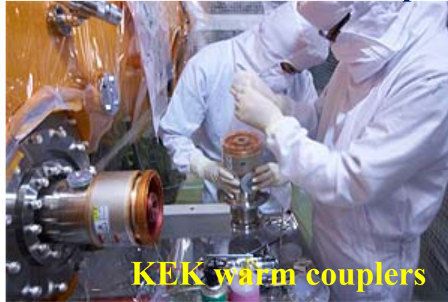
Assembly of DESY/FNAL/KEK warm couplers
