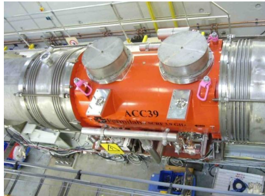
■ The 3.9 GHz FLASH accelerator module as prototype.
