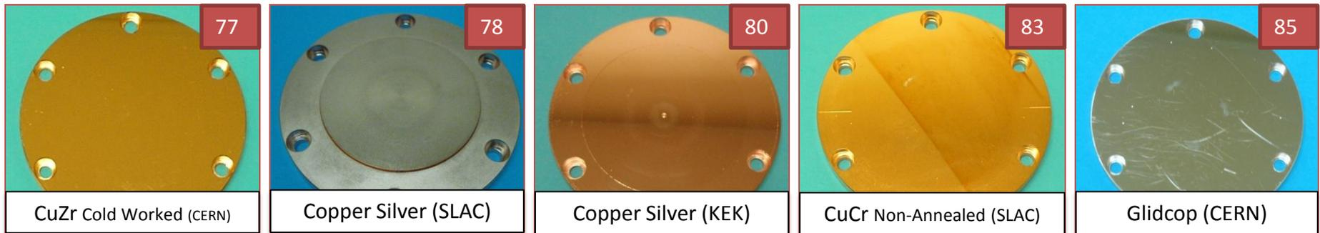
Breakdown and pulsed heating effects on an standing wave accelerating structure iris
