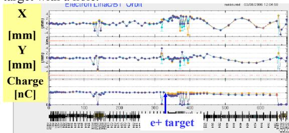
Figure 13: Machine study result of the new positron target. The horizontal (upper), vertical (middle) beam orbit and beam charge (bottom) are shown along the linac. The blue and orange dots mean the results of original and new scheme, respectively.
