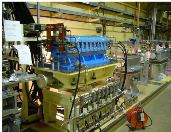
Figure 10: Photograph of the pulsed bending magnet for the new PF-BT.
