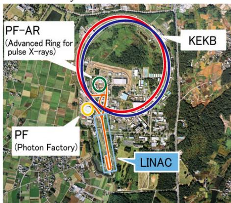
Figure 1: Accelerator complex in KEK Tsukuba campus.
