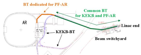
Figure 14: Schematic drawing of BT for KEKB and PF-AR.
