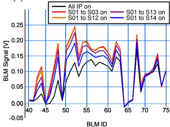
Figure 4: BLM raw signals with different IP settings. With all IP's on (black), IP's from SDTL04 to SDTL15 off (red), IP's from SDTL13 to SDTL15 off (orange), IP's from SDTL14 to SDTL 15 off (purple), and IP of SDTL15 off (blue). BLM #40 corresponds to the one at the SDTL end, and BLM #44 to #60 corresponds to those in the future ACS section.
