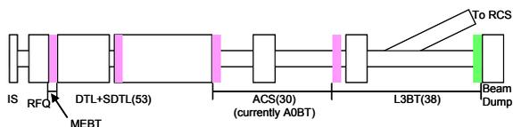
Figure 1: Layout of J-PARC linac and location of WSM. Pink boxes are the matching sections and green box is a place where the WSM with beam size monitor is installed. Brackets are the numbers of BLM in each section.
