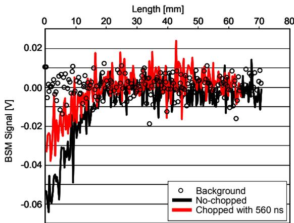
Figure 6: Signal from  $H^0$  particles taken by carbon plate. Circle dots are signals taken under no beam operation. Signal from  $H^0$  particles with no-chopped beam is indicated with black line. Signal from  $H^0$  particles with chopped beam with about half duty of no-chopped beam is indicated with red line.
