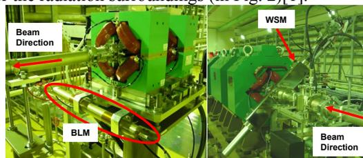
Figure 2: Installation of the BLM and WSM are shown. BLMs are installed behind the quadrupole magnet (left). WSMs are installed at the upstream of the matching section (right).
