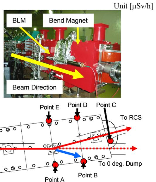
Figure 5: Measurement for residual radiation around the first bending magnet in L3BT section. BLMs are installed at the both sides of the bending magnet (top-left). Points A to E are the measurement point for residual radiation (top-right). Main beam orbit is along with the red line, orbit of the remained proton ( $H^+$ ) is blue line.
