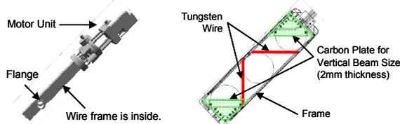
Figure 3: WSM and its frame are shown. Wire frame (right) is connected to a shaft controlled by motor unit and it is installed in a vacuum chamber (left).
