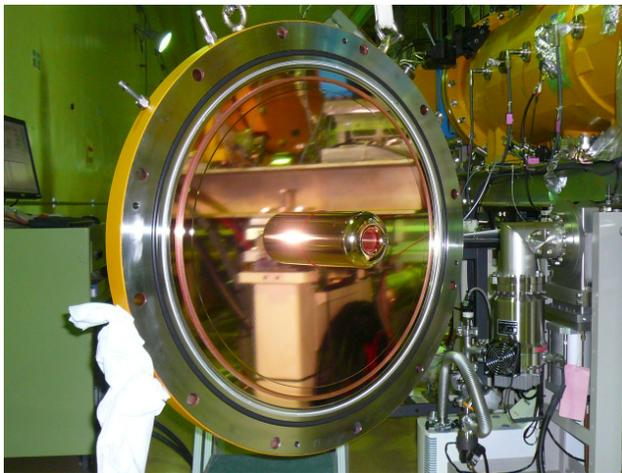
Figure 4: The end plate detached from the SDDL. The inner seal (silver) is an E-seal and the outer seal (black) is an elastomer O ring.
