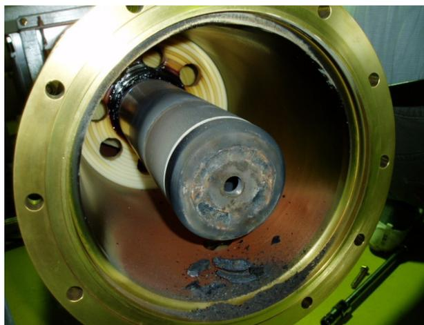
Figure 3: Photograph of damaged coaxial tube.
