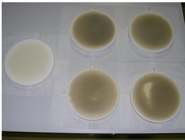
Figure 2: Photograph of the ceramic window. The left one is an unused window and four other windows are used.
