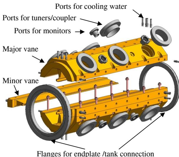
Figure 1: Schematic drawings of the vanes of the unit tank.
