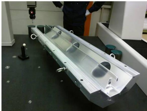
Figure 2: Aluminium test milling cut model.
