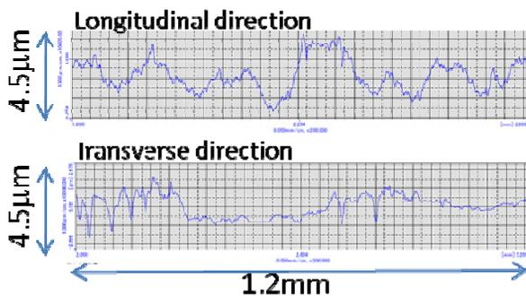
Figure 3: Top: is a close-up photo of the vane tip. The material of this TP is annealed oxygen-free copper. The cutter mark left by the ball-end-mill machining can be clearly seen. Bottom: trace is the measured surface roughness of the vane modulation. Typical surface roughness is 0.8µm.
