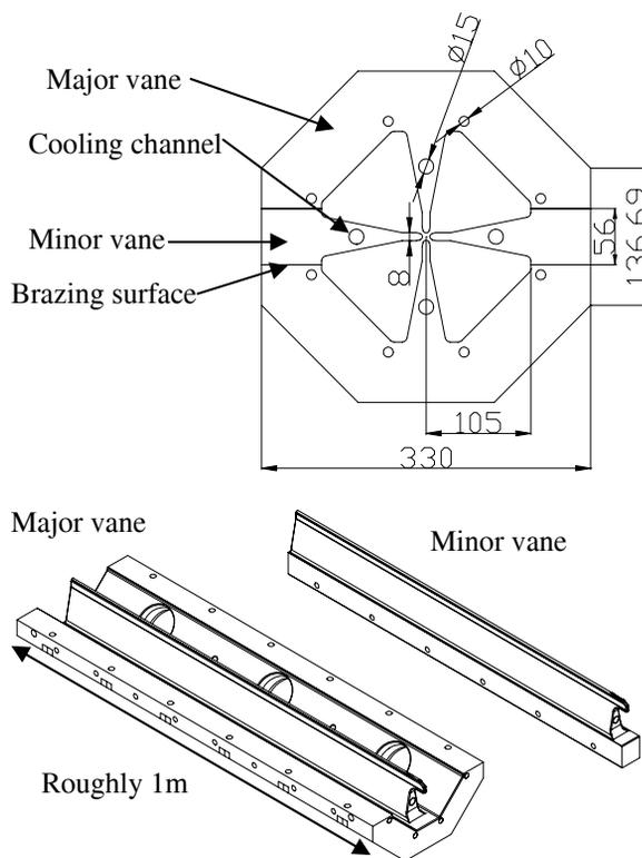
Figure 1: Schematic drawings of the unit tank vanes. The cooling channel was machined by gun-drill and plugged by electron beam welding.
