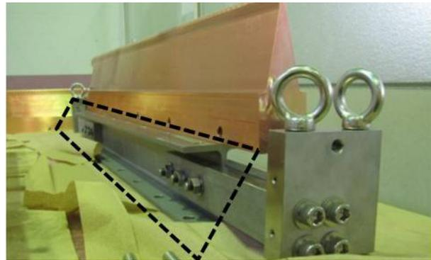
Figure 7: Vanes are bolted on the backbone during the transportation.
