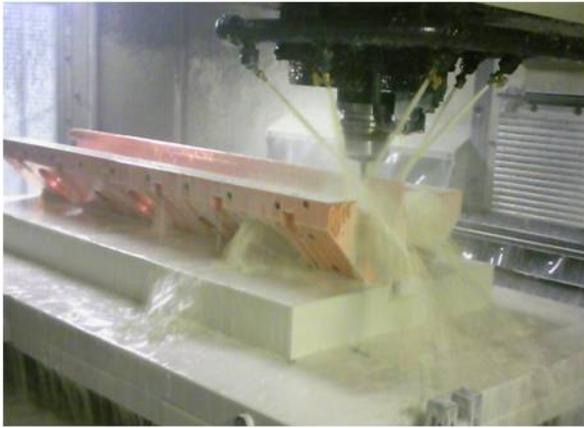
Figure 5: Ball-end-mill machining of the RFQ modulation.
