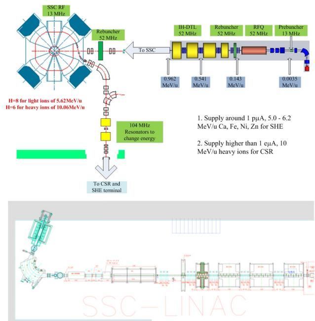
Figure 1: Conceptual design of SSC-LINAC.
