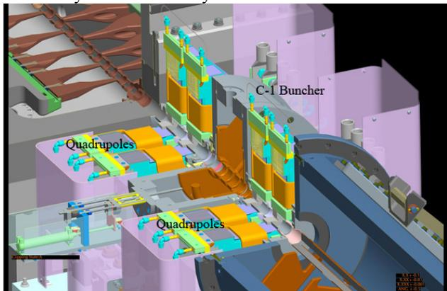
Figure 5: Cross-sectional view of the MEBT section.
