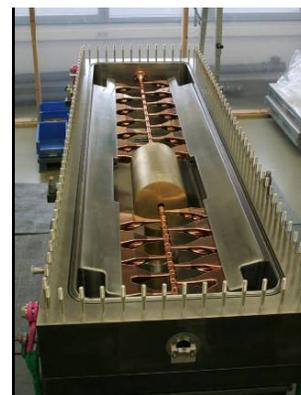
Figure 2: IH linac during initial rf testing at IAP Frankfurt, Germany.
