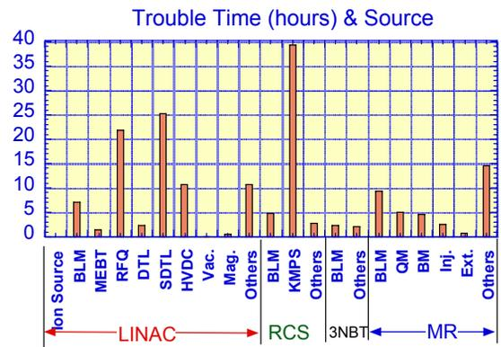
Figure 3: Beam down time by major subsystems.
