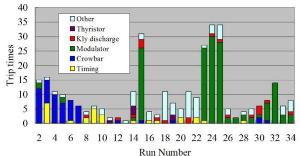
Figure 4: Number of trips related to high power RF components.
