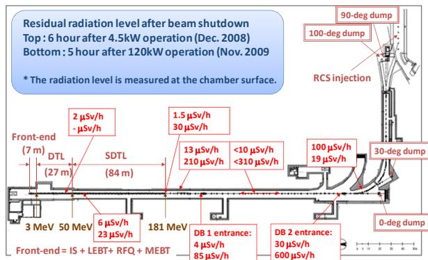
Figure 5: Residual radiation level after the beam shutdown for 4.5 kW and 120 kW @3GeV cases.
