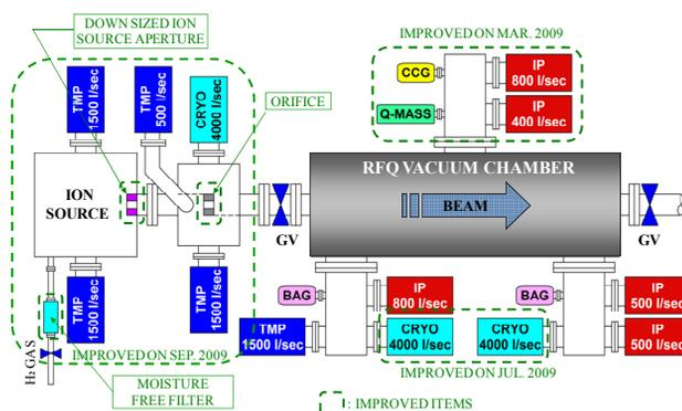
Figure 1: Vacuum system at the front end.
