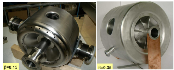
Figure 13: 352 MHz, \beta=0.15 and 0.35 single-spoke cavities developed for the EURISOL and EUROTRANS projects [15, 19, 20].
