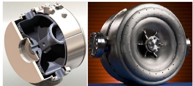
Figure 14: Present concept for Fermilab's Project X (upper), concept for the cw linac (middle), and prototype of the 325 MHz, \beta=0.22 single-spoke cavity.
