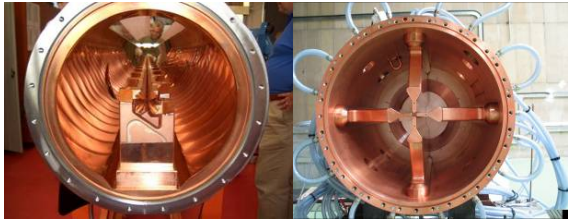
Figure 3: Front view of the SARAF RFQ (176 MHz four rods) and SPIRAL2 RFQ (88 MHz four vanes).
