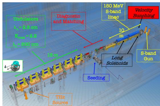
Figure 4: The SPARC Accelerator layout
