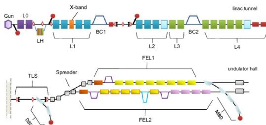
Figure 1: Split schematic of FERMI@Elettra, including the S-band linac, the X-band cavity, the bunch compressors (BC1 and BC2), transfer line (TLS, spreader), FEL lines and beam dumps (DBD, MDB).
