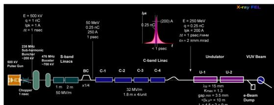
Figure 8: SCSS test accelerator schematic view
