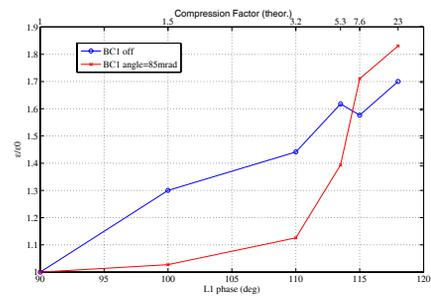
Figure 2: Relative emittance growth in BC1 area, with and without compression. The error on the central values is of the order of 10%
