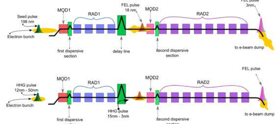
Figure 3: The HGHG scheme for FEL 2 (on the top) and the compatible HHG-seeding scheme (on the bottom) [10]
