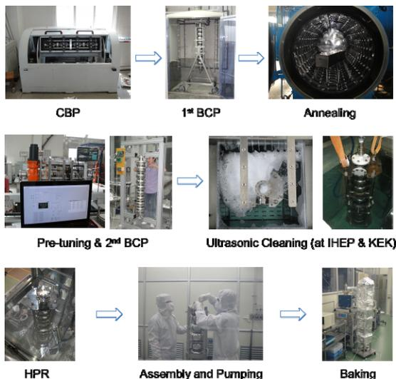
Figure 2: Surface processing for IHEP-01 cavity.
