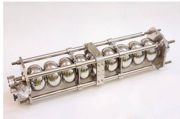
Figure 1: IHEP-01 large grain 9-cell cavity.
