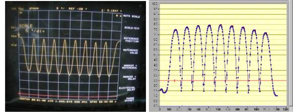
Figure 3: IHEP-01 9-cell cavity field flatness before (94 %) and after vertical test (90 %).
