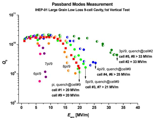
Figure 5: Passband test results of IHEP-01.
