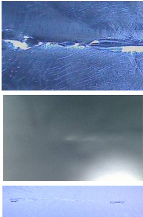
Figure 6: Cell #9 equator 270-300° as delivered(top), after final CBP (middle) and the 1<sup>st</sup> vertical test (bottom).
