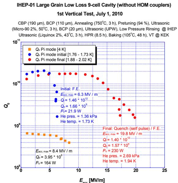
Figure 4: Test result of the IHEP-01 large grain los-loss shape 9-cell cavity (without HOM couplers).
