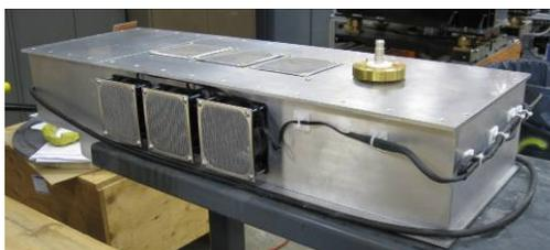
Figure 4: Isolation transformer.
