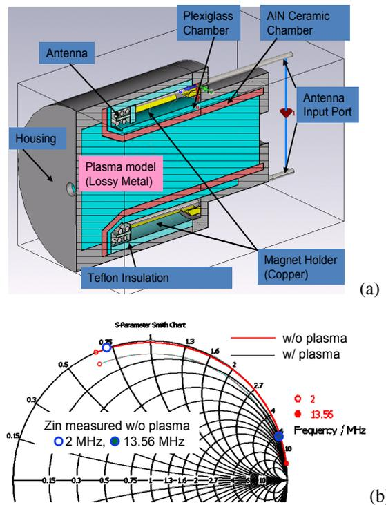
Figure 1: (a) External antenna ion source, (b) computed input impedance of the external antenna.
