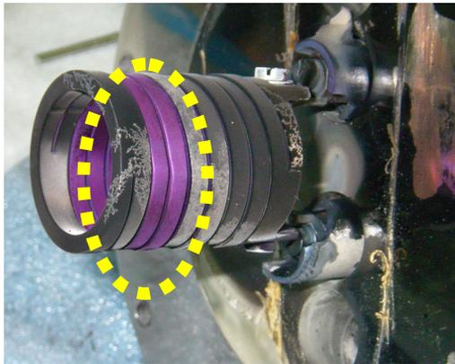
Figure 3: Photograph of the LaB<sub>6</sub> filament after approximately 600 hours operation.
