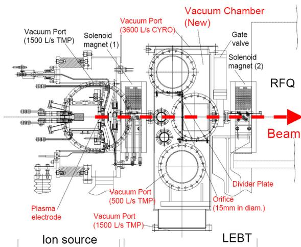
Figure 2: A schematic drawing of the new configuration of the LEBT.
