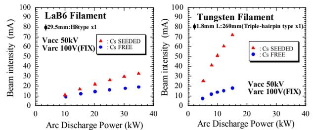
Figure 4: Dependence of H<sup>-</sup> ion current on arc discharge power driven with LaB<sub>6</sub> or W filament for Cs-seeded and Cs-free condition.
