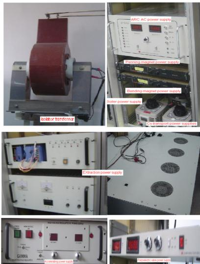
Figure 3: Main power supplies for ion source.
