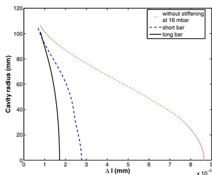
Figure 2: ANSYS™ simulations of backwall deformations at 1.8 K, 16 mbar and cavity under vacuum for various stiffening configurations (Note that the final spider configuration is better than the long bar but is not shown). The abscissa depicts the longitudinal deformation and the ordinate the cavity radius from the cathode region to the equator of the 0.6 cell.
