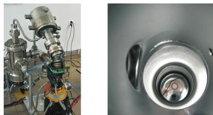
Figure 3: Left: Setup at Swierk for plasma arc deposition of the lead cathode in a 30° configuration between source and deposition target area. Right: Picture of the inner cavity surface after deposition of the lead cathode. The cathode is visible as a greyish spot in the middle of the backwall next to the visually emphasized grain boundary.
