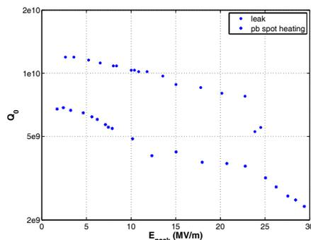
Figure 5: Cavity vertical tests after the lead coating and further cleaning. The blue dot curve shows a test where a vacuum leak occurred. The second test with sealed conditions showed a degradation of  $Q_0$  with the field and also the temperature at the cathode position was abnormally high.
