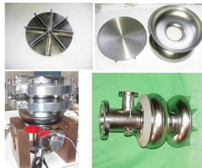
Figure 1: Top left: Cathode backwall with “spider” stiffening bars, top right: Cavity half-cells and large grain Niobium backwall, lower left: Cavity tuning setup at JLab, lower right: Fully assembled cavity with helium vessel endplate and coupler ports.
