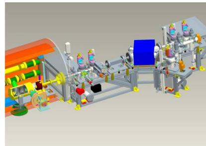
Figure 6: Setup of the gun cavity in the HoBiCaT cavity test facility and the new diagnostic beamline.
