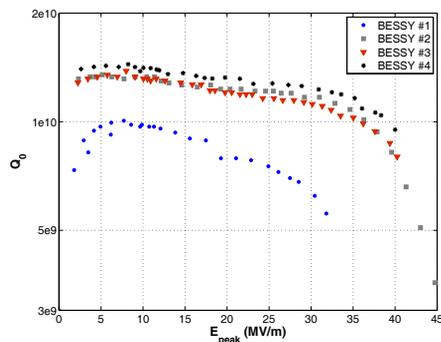
Figure 4: Cavity vertical tests after assembly (#1), further tuning and cleaning (#2), after following installation of the helium vessel (#3) and after loss of the lead cathode and removal of remnants by grinding and BCP (#4).
