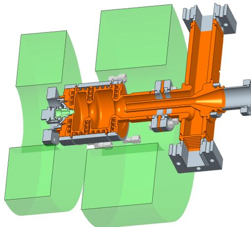
Figure 1: Gun section layout. It consists of a gun and a coupler. An exchangeable cathode is installed at the rear wall of the gun. The connecting parts to other vacuum components and RF window are shown. The focusing solenoids are also shown.
