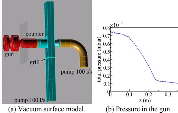
Figure 7: Vacuum simulation. The simulation shows the total pressure on the symmetry axis of the gun. The cathode is at  $z = 0$ .
