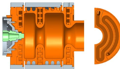
Figure 2: A cut view of the gun body (left) and a half of the cooling channel in the irises and rear wall (right). There are 8 water inlets and 8 outlets in total.
