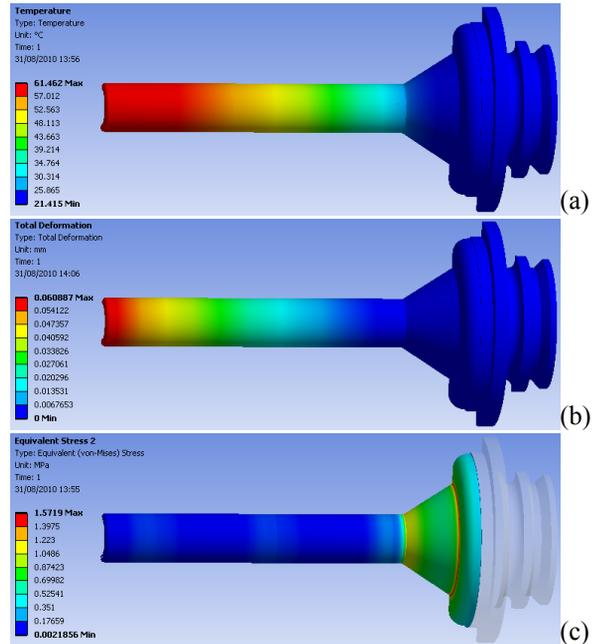
Figure 6: Steady state temperature (a), deformation (b), and stress (c) at the coupler inner antenna.
