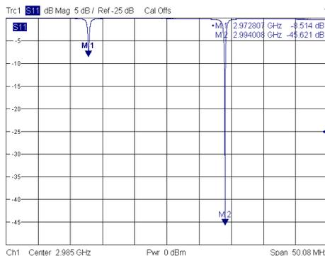
Figure 9: S11 measurement with a network analyzer.
