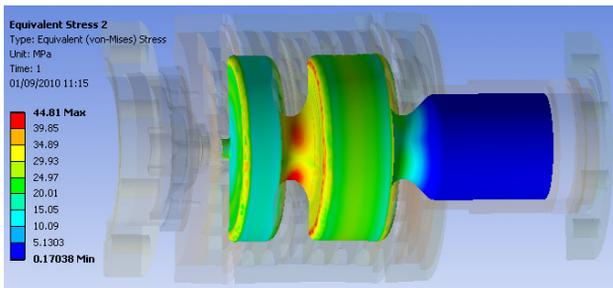
Figure 5: Steady state von Mises stress on the RF surface of the copper body.
