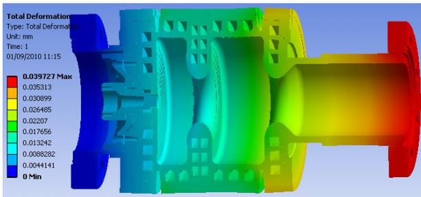
Figure 4: Cavity deformation caused by the RF heating.
