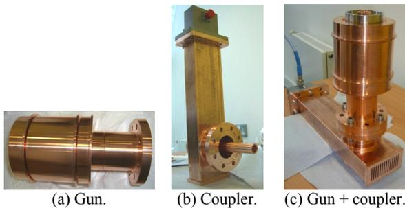
Figure 8: Constructed prototype for cold test.
