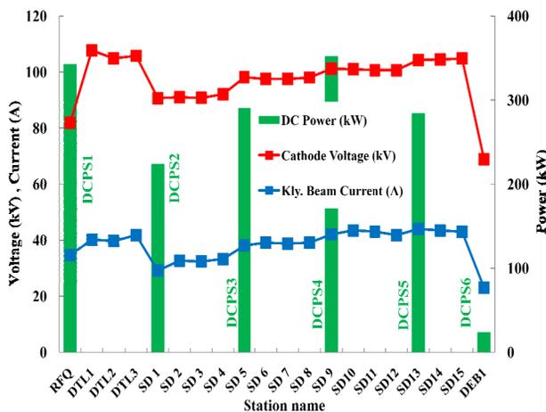
Figure 4: The Sample data of 181 MeV linac, operating on June 28, 2010. DCPS5 drives three klystrons (SDTL13-15), and DCPS6 drives one 324MHz klystron (DEB1).
