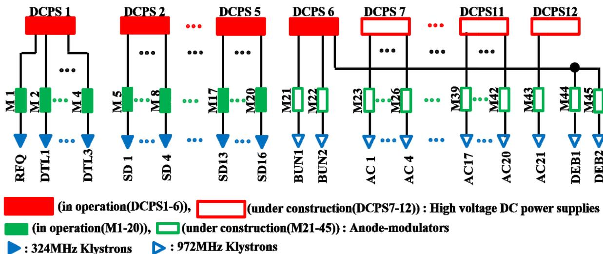
Figure 1: Configuration of power supply system for klystrons in J-PARC 400MeV linac.
