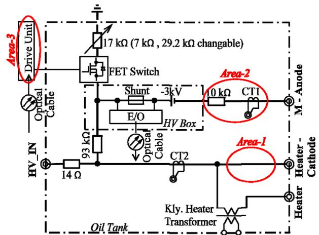
Figure 2: Schematic diagram of anode-modulator (M1-20).
