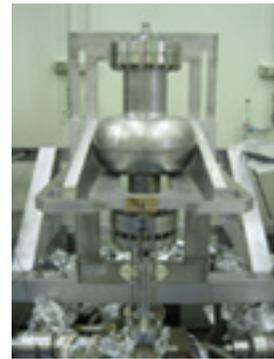
These cavities were surface treated initially by buffered chemical polishing (BCP). Just HPR and short baking took place for the successive cold tests. Gradients were most likely limited by Q-slope or field emission.
