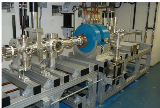
Figure 1: The new AWA RF gun (between the blue solenoids) is being commissioned, initially with a copper photocathode, which will soon be replaced with a Cesium Telluride photocathode. This gun will replace the present drive gun as the source of drive bunches.
