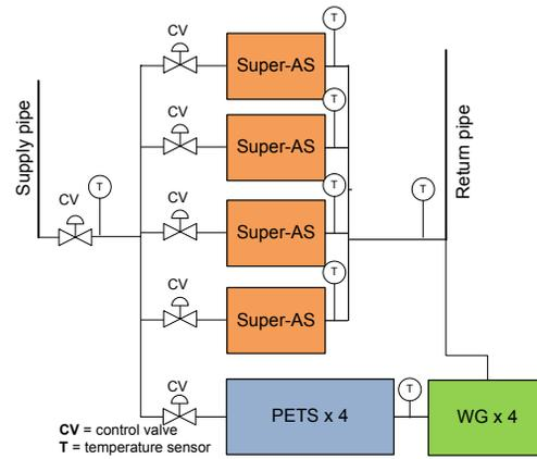
Figure 2: The TMM cooling water distribution; Super-AS: two consecutive accelerating structures; WG: waveguide.
