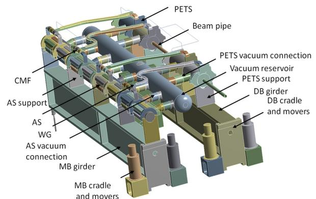
Figure 1: Thermo-mechanical model configuration based on a typical CLIC module type.
