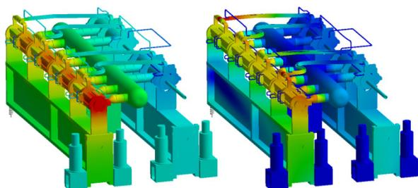
Figure 3: Temperature (left) and deformation (right) contours for unloaded condition including vacuum and gravity load conditions; Red: large variation, Blue: small variation.
