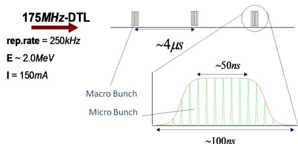
Figure 2: Proton pulse structure at the entrance of the ARMADILLO.
