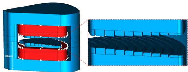
Figure 6: Preliminary design of the duplex-gradient dipole.
