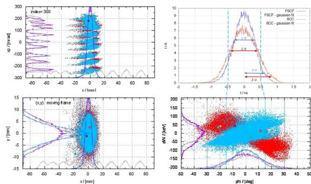
Figure 8: Merging: Projections at the Li-target. Transport with *Full Space Charge Forces* (FSCF, red and violet) compared to *Space Charge Compensated* (SCC, blue) transport. The longitudinal coordinate  $\phi$  is given by the rf-phase at 87.5 MHz. Grey lines are the initial beam profiles, when merging is started.
