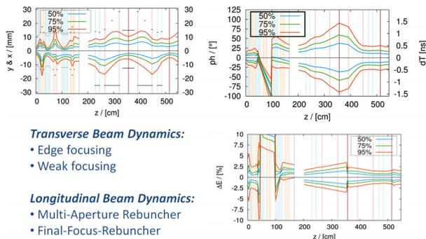
Figure 7: PSO-result for the central trajectory. The transverse dimensions of the micro bunch are significantly smaller than the given apertures (black bars). In principle a 1ns micro bunch with an energy spread less than  $\pm 5\%$  is possible at the exit of ARMADILLO.
