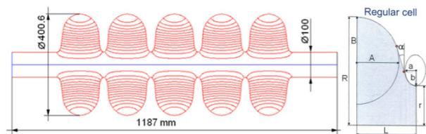
Figure 2: Layout of the  $\beta = 0.9$  five-cell cavity.
