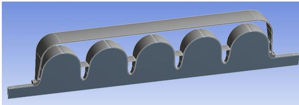
Figure 5: An RF/mechanical model to assess the df/dP.
