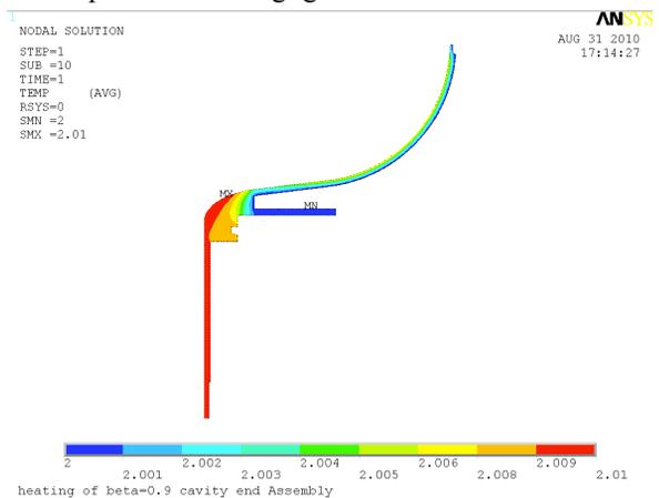
Figure 6: Thermal distribution at the end cell.
