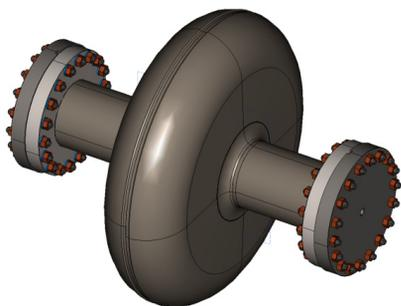
Figure 3: Layout of a  $\beta = 0.61$  single-cell cavity.
