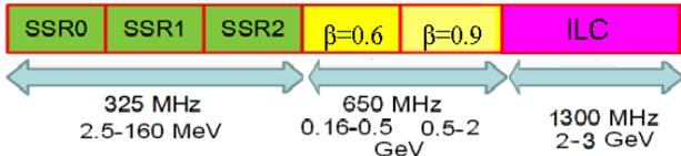
Figure 1: Layout of the Project X superconducting Linac.
