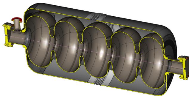
Figure 4: Layout of a  $\beta = 0.9$  five-cell cavity with vessel.
