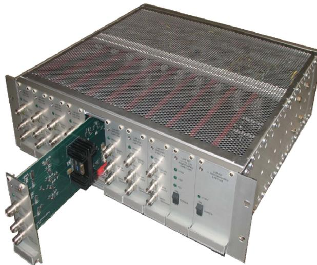
Figure 3: Piezo Tuner amplifier chassis
