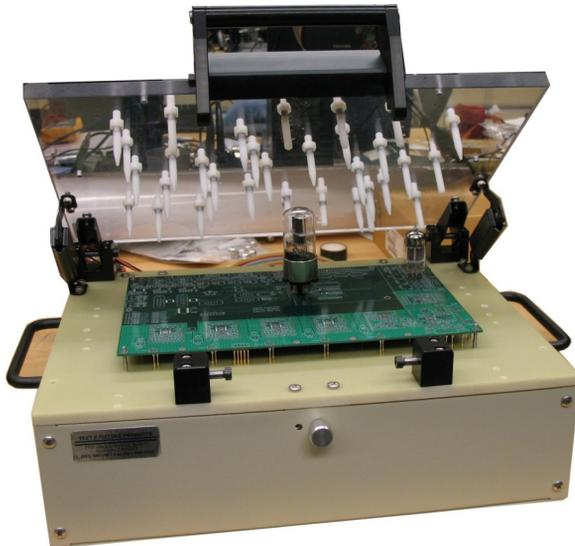
Figure 4: Digital board "bed of Nails" test stand
