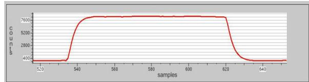
Figure 6: Pulsed waveform of the cavity transmitted power. The vertical scale is ADC counts and the horizontal is samples where one sample is 1.17 ms. Cavity gradient was 7 MV/m.
