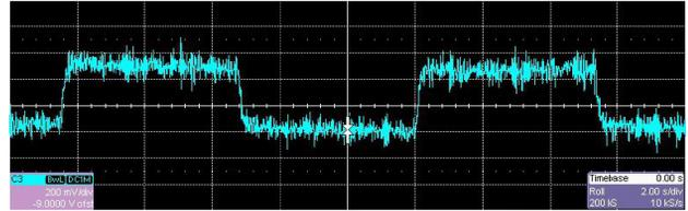
Figure 5: Field Control Chassis diagnostic output (DAC) of the detectable tuning resolution. Cavity was tuned back and forth in 1 Hz steps using the stepper motor.
