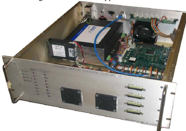
Figure 2: Stepper motor control chassis
