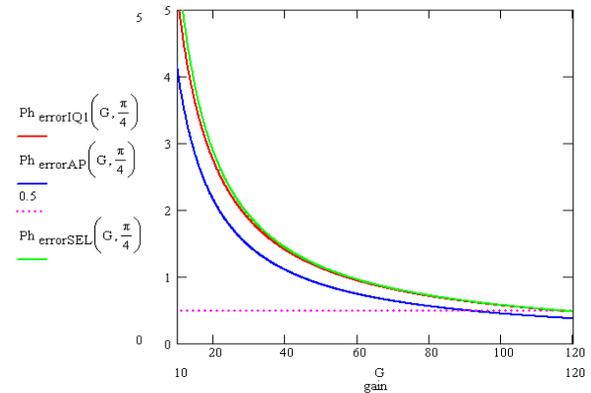
Figure 5: Phase error versus regulation gain  $G$  for I&Q Amplitude&Phase and SEL architectures.
