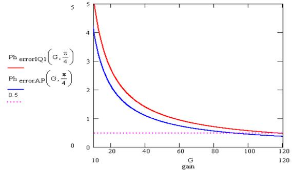
Figure 3: Phase error versus regulation gain  $G$  for I&Q and Amplitude&Phase architectures.
