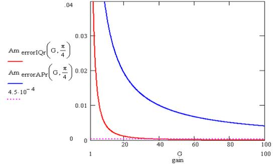
Figure 2: Relative amplitude error versus regulation gain  $G$  for I&Q and Amplitude&Phase architectures.
