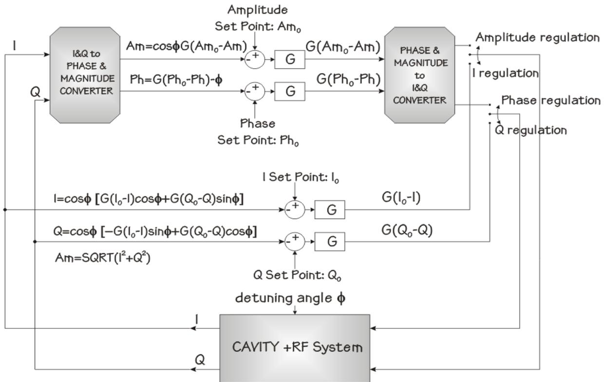
Figure 1: Amplitude&Phase versus I&Q regulation architecture.
