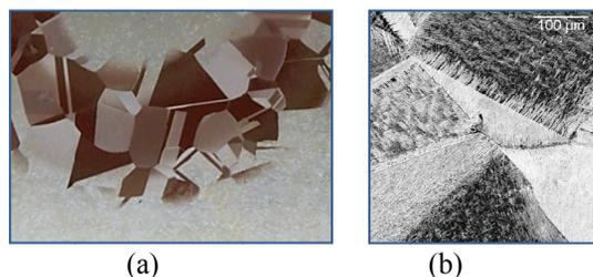
Figure 4: (a) SPDT Cu sample and (b) HIP Cu sample with neighboring grains having varying degrees of surface damage.
