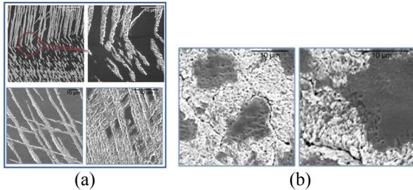
Figure 5: (a) Transgranular extrusions oriented in different directions and terminating along grain boundaries creating a weave-like pattern and (b) extrusions through micropits.
