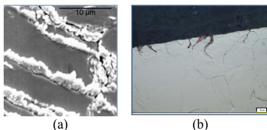
Figure 2. (a) SEM images showing surface extrusions on copper sample tested to 110°C. (b) Metallography showed subsurface damage along grain boundaries extending 20-40µms below the surface.
