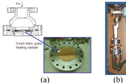
Figure 1: (a) Pulsed heating cavity with 3" sample attached to cavity end cap and (b) connected to power source through a  $TE_{10}$  (WR90) to  $TE_{01}$  mode converter.
