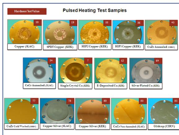
Figure 3: Pulsed heating samples that were tested to 110°C shown in order of their material hardness.
