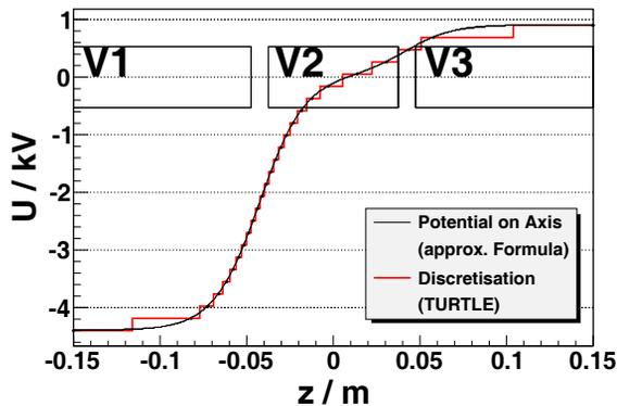
Figure 5: Potential on the axis of the einzel lens. The tube voltages have been chosen according to the operating parameters for <sup>4</sup>He (V1 = -4.4 kV, V2 = 25.0 V, V3 = 0.9 kV).
