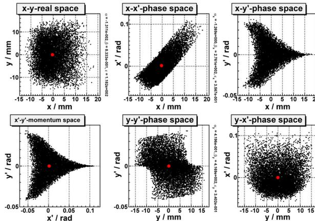
Figure 6: Particle distribution at the position of the profile grid.
