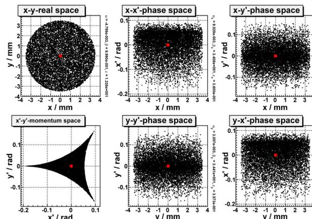
Figure 4: Particle distribution at the plasma lens of the ion source. The centre of mass is marked with a red dot.
