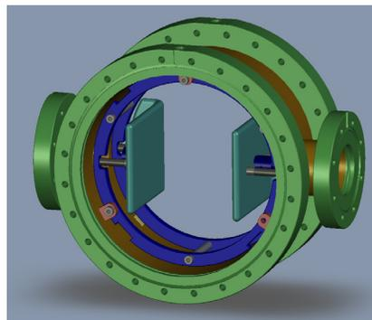
Figure 3: 3D model of the new macro-pulse chopper.
