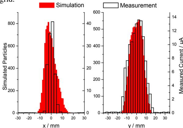
Figure 7: Simulated and measured beam profiles at the position of the profile grid.
