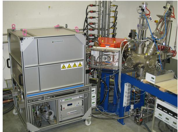
Figure 1: Current test bench setup with ion source (left), analyser dipole (centre) and beam diagnostic chamber (right; with slit, profile grid and Faraday cup).
