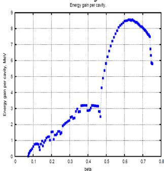
Figure 2: Energy gain for the initial cavities of the proposed Fermilab SRF Project-X CW Linac. The beta=1 part of the linac would have ~17 MeV/m.
