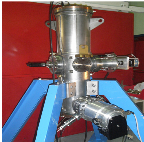
Figure 1: The RF cavity prototype on its test bench for characterisation before reception.
